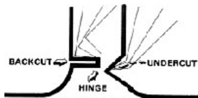
Figure 5. Each tree felled requires first an undercut done on the side to which the tree will fall, and then a backcut. Be careful to leave a "hinge" of uncut wood.
