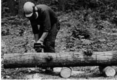
Figure 7. Identifying the location of tension and compression wood in a trunk will make it easier to buck without binding the saw bar.
