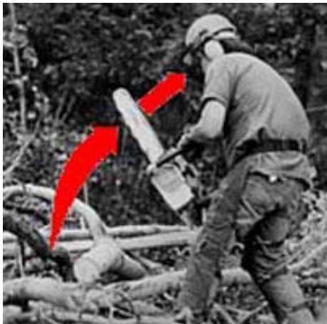
Figure 2. A kickback can occur in less than one-tenth of a second, faster than the human brain can respond.
